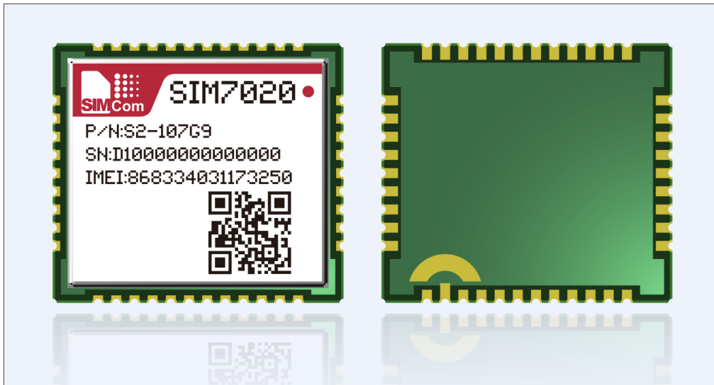
Figure 25: Top and bottom view of SIM7020
